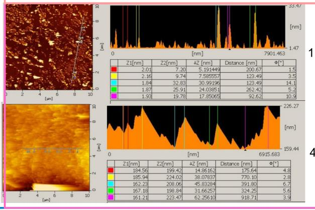
Growth of the layer can constated through the difference of height between the 1L and <sup>40L</sup>40L thin films.
