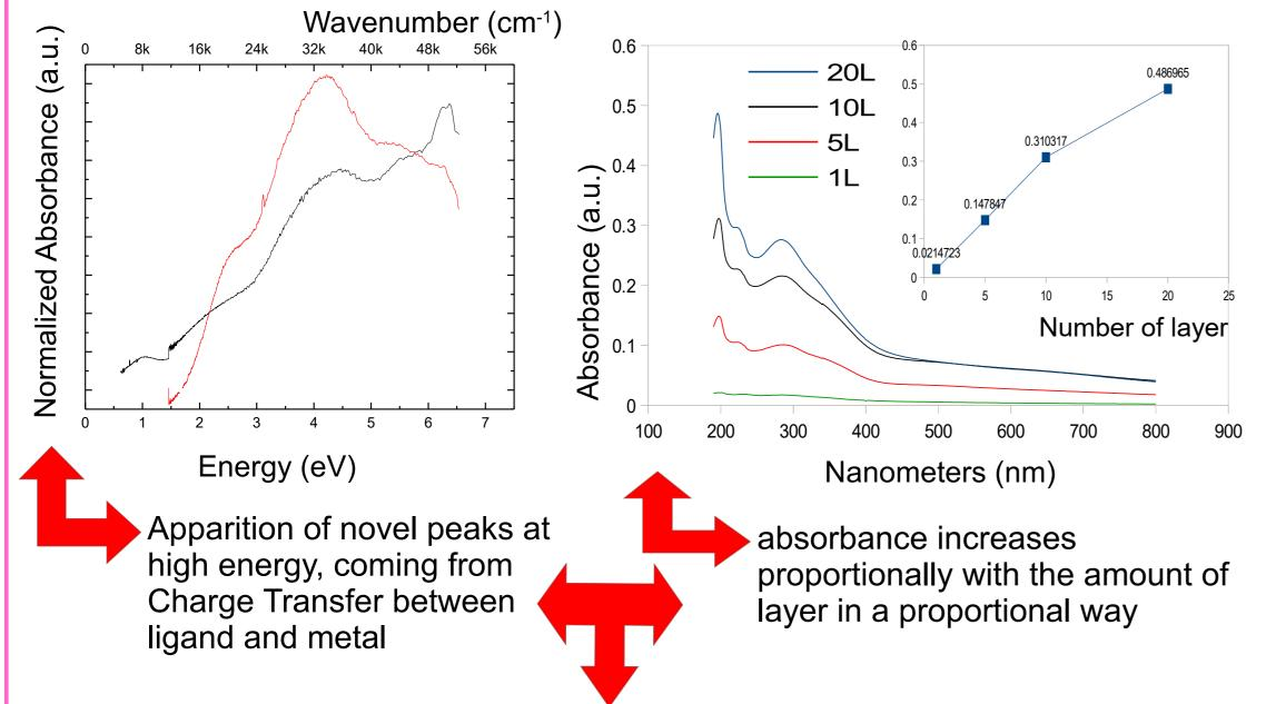
Coordination of organic ligand with metal is proven through the apparition of Charge Transfer and control of the growth of the thin film through LbL is validated with **Beer-Lambert law**
